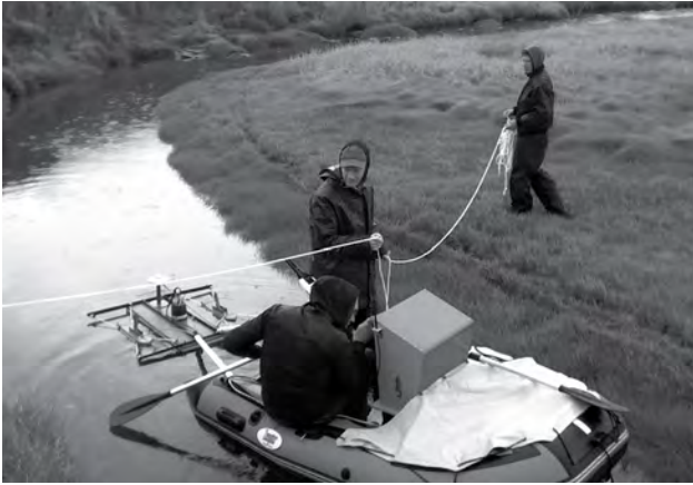
Leiruvogur harbor is frequently mentioned in the Icelandic sagas, but its original location was unclear. MAP collaborators used a specially built seismic refraction array (above), ground penetrating radar, and electrical resistance tomography to identify the Viking Age harbor's borders.
